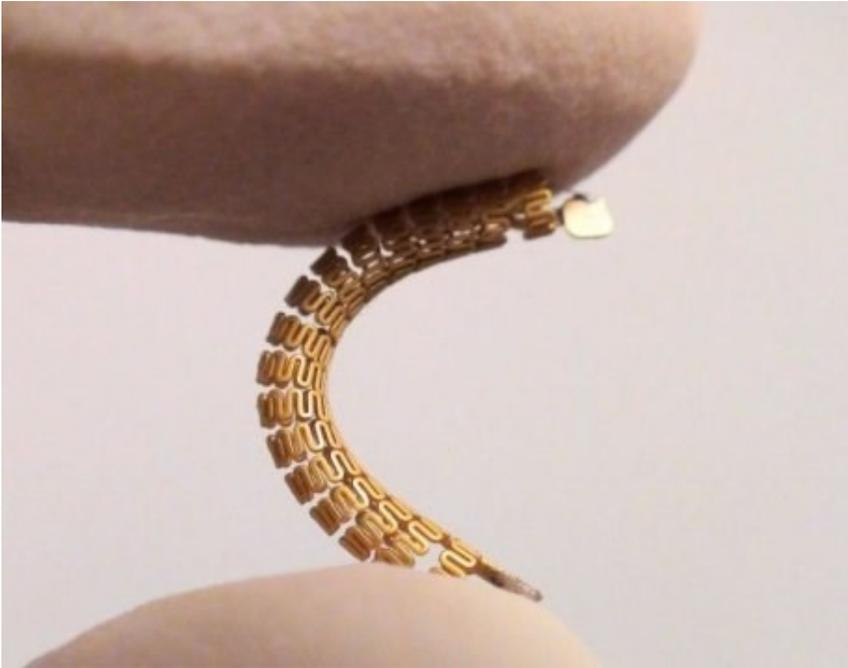
Now, a team led by UBC electrical and computer engineering professor Kenichi Takahata has developed a type of "smart stent" that monitors even subtle changes in the flow of blood through the artery, detecting the narrowing in its earliest stages and making early diagnosis and treatment possible.
